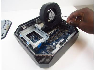
• Carefully disconnect the CPU fan by pulling out the wires from the motherboard.
