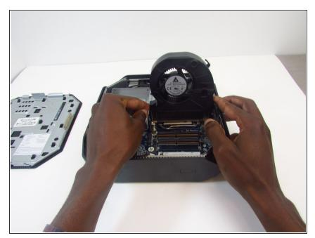
Swing the fan upward, to a 90degree angle.
