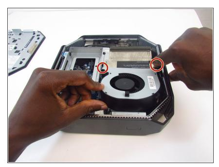
Swing the fan back down and carefully unhook the CPU fan notches by pulling each tab away from the heat sink holes.
