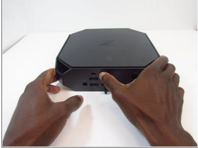
Slide and hold the latch in the direction of the engraved arrow (to the right).
