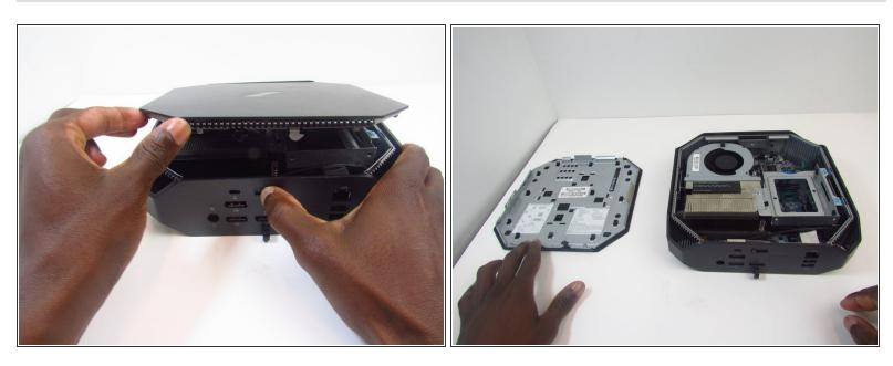
While holding the latch, lift the access panel upwards and towards yourself and set it aside upsidedown.
