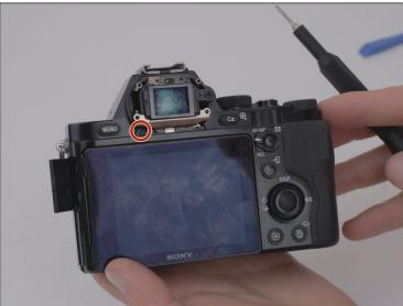
• Remove the four M 1.5x2mm screws.
