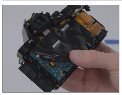
Peel off the large black protective adhesive from the motherboard.
