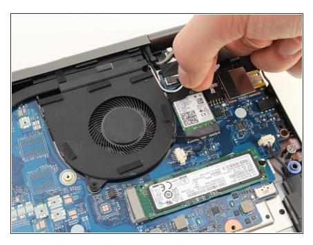
Remove the sticky tape from the top edge of the wireless card.
