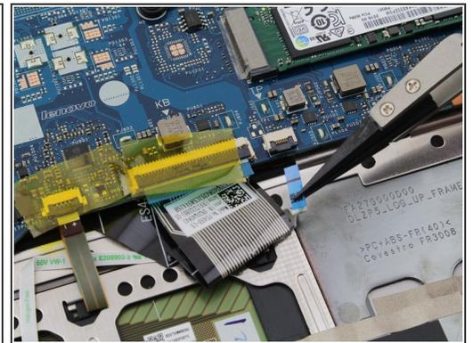
**i** The touchpad is connected by a ribbon cable to the front edge of the motherboard.
