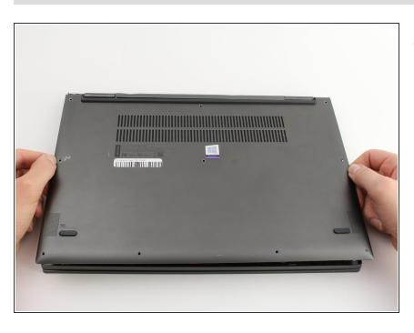
Pull the bottom cover up and away from the back hinges.
