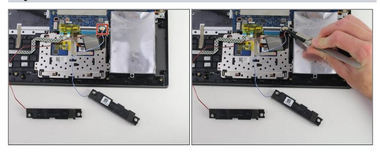
• Carefully unplug two wired connections from the motherboard using nylon tip reverse <u>tweezers</u>.
