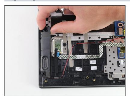
Remove the two speakers from their compartment. The speakers are held in the bottom corners of the device.
