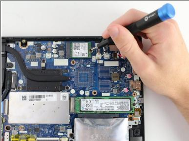
• Using the Phillips #00 screwdriver, remove one 3.6 mm screw.
