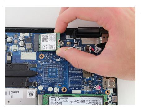
Remove the wireless network adapter.
