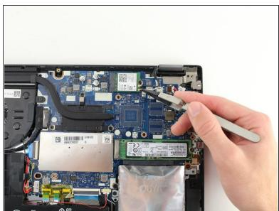
Use the reverse tweezers to carefully unplug the two wired connections.
