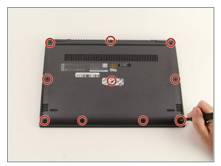
Remove all ten 6.6 mm screws with a Phillips #00 screwdriver.
