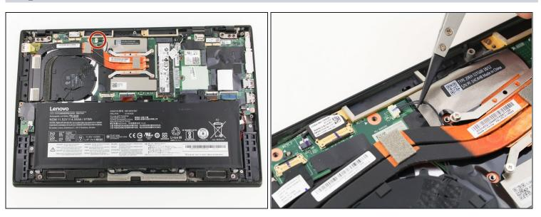
• Use nylon tipped tweezers, or your fingers, to gently pull the fan's power cable towards the SSD, disconnecting it from the pins.
