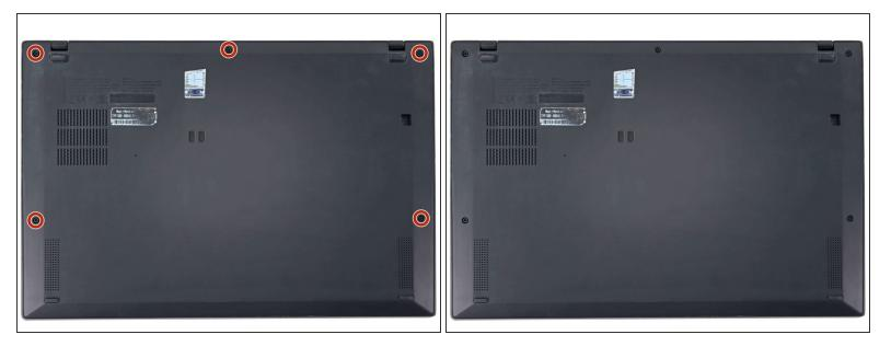
• Use a Phillips #1 screwdriver to loosen the five captive screws securing the back cover.
