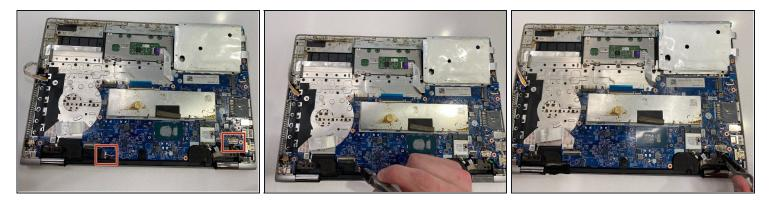
• Use the Reverse <u>Tweezers</u> to disconnect the speaker cables from the motherboard.
