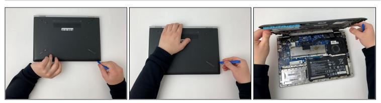
• Using the opening tool, carefully remove the bottom cover from the device.
