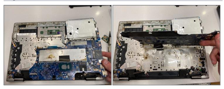
• Gently lift the motherboard out of the device
