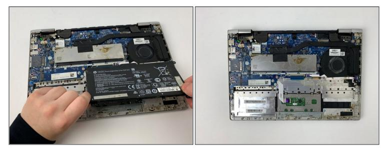
• Carefully lift from the base and remove the battery.
