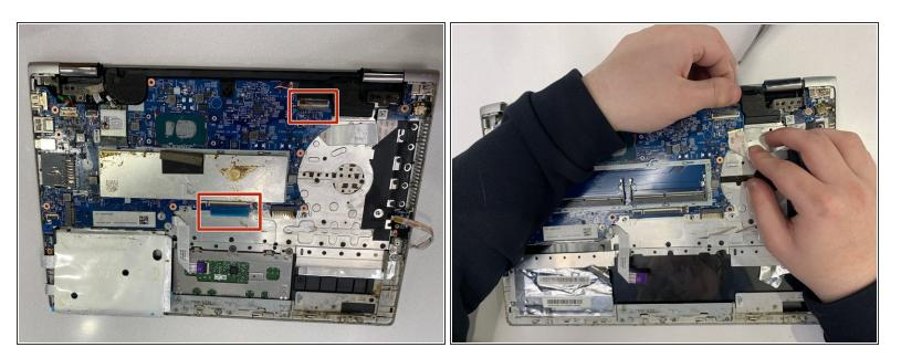
• Grab the ribbon wires by the edge of the socket and pull to remove them from the motherboard.
