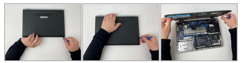
• Using the opening tool, carefully remove the bottom cover from the device.
