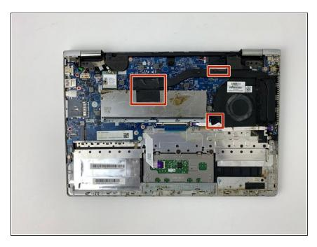
• Remove the tape that secures the fan to the computer.
