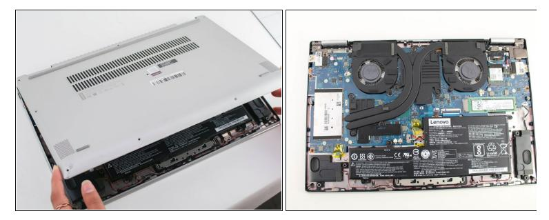
• Pry around the edges from one side to another with a plastic opening tool.
