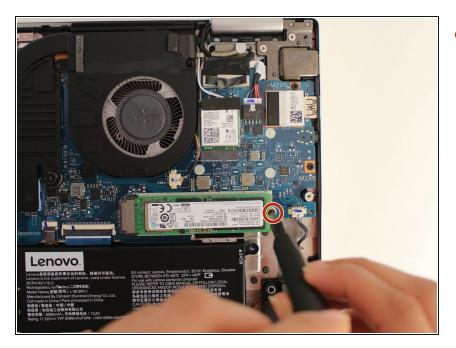
Remove the one JIS #1 screw holding the SSD.
