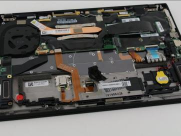
• Peel back the black adhesive tape covering the ribbon cable connecting the trackpad and fingerprint scanner to the motherboard.
