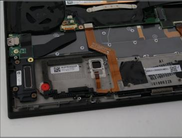
• Using an opening tool, lift the fingerprint scanner upwards.
