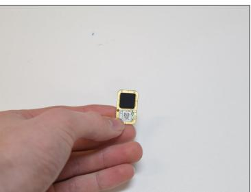
• Carefully lift the fingerprint scanner to remove from the chassis.
