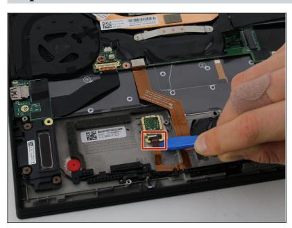
Unclip the connector ribbon from the fingerprint scanner by lifting upwards on the clip with an opening tool.
