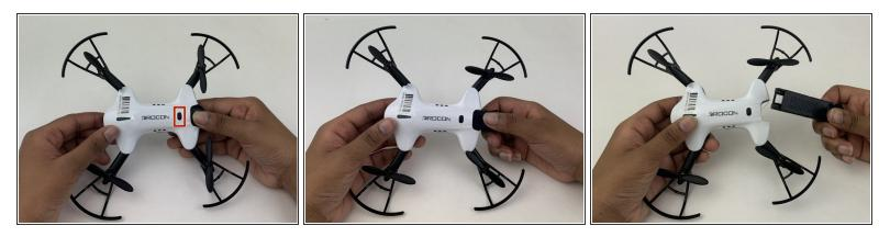
Make sure the drone is powered off before beginning the battery replacement.
