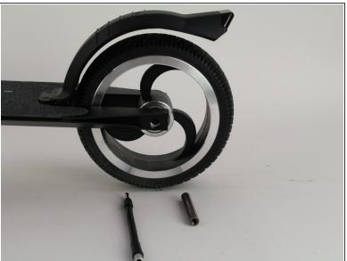
Use a 4 mm bit extension to push the axle out of the wheel's center.
