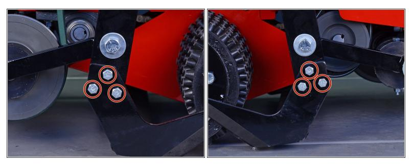
Use a 1/2" socket wrench to remove the six 1 inch-long bolts securing both ends of the blade. You may need to use a 1/2" combination wrench to hold the nuts in place.
