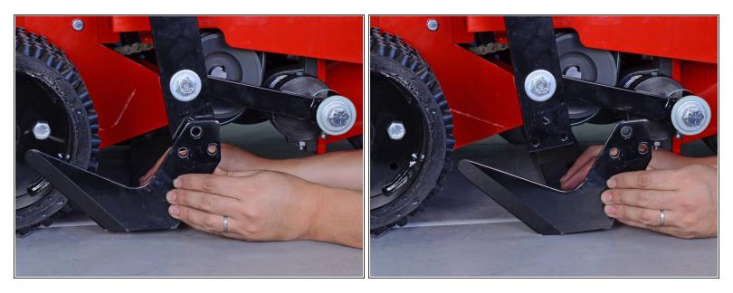
The blade can be very sharp! Do not handle the blade from the cutting edge.
