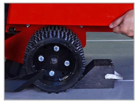
• Place wheel chocks against the roller and rear wheel to prevent the machine from moving.
