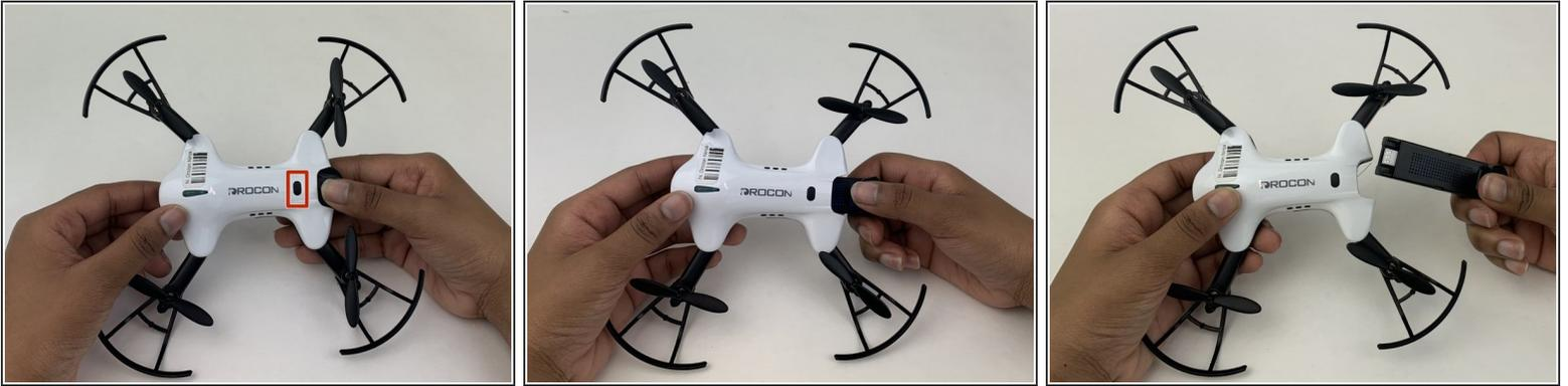
**⚠** Make sure the drone is powered off before beginning the battery replacement.
