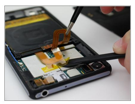
Slowly slip the halberd spudger underneath the rest of the orange flex cable to carefully peel the adhesive portion away from the rest of the phone.
