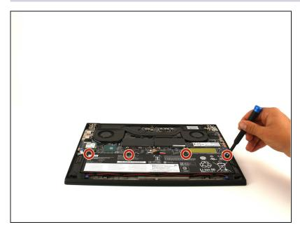
Use a Phillips #00 head screwdriver to remove the four 4 mm screws above the battery.
