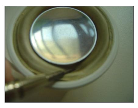
Sometimes, the cone also gets unglued from the rubber ring. The procedure is the same - use contact glue. Put everything back together, following the steps in the reverse order: gently pull the wire in the back of the housing (allow some loose wire inside the housing, don't let it too tight), put the driver in it's place and put the screws back.
