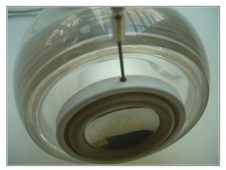
Using a small Philips screwdriver, gently unscrew the 3 screws sitting around the speaker (if yours have a grill, remove it, first.
