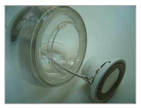
• In order to make some room to work, it's necessary to pull some wire off. Pinch the wire inside the housing with two fingers and (again) gently pull it some 2-3 inches. It's not easy, but it will come out, little by little. A small amount of silicone spray in the metal ring, in the back of the housing (where the wire comes in) may help.
