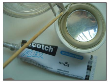
Use a small amount of contact glue. I used a thin wood stick as a tool. Follow the glue instructions. The picture shows a small piece of carton paper holding the rubber, while glue is applied.
