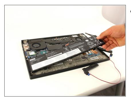
Lift the battery out of the frame and remove it from the device.
