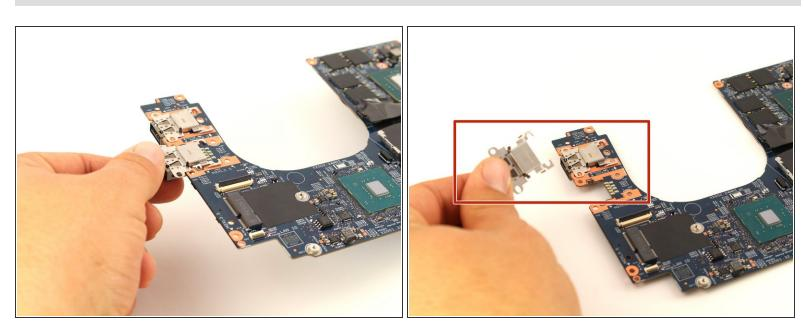
Gently push the docking station towards the center of the motherboard, lift up to release a lock, then pull it out to remove it from the device.
