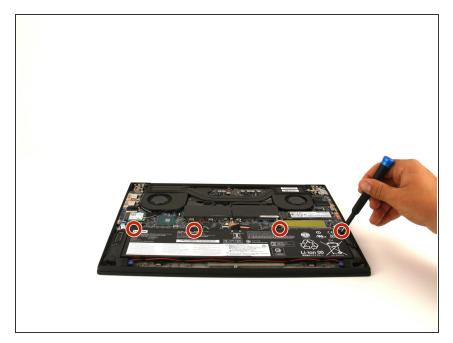
Use a Phillips #00 head screwdriver to remove the four 4 mm screws above the battery.
