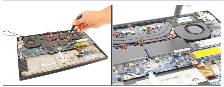
• Loosen the five screws connecting the fan to the motherboard using a Philips #00 head screwdriver.
