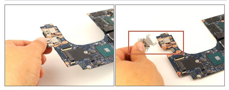
• Gently push the docking station towards the center of the motherboard, lift up to release a lock, then pull it out to remove it from the device.
