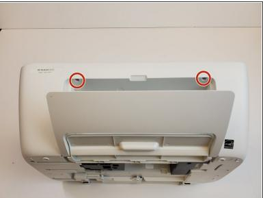
Using the Torx T5 screwdriver, remove the four screws connecting the scanner bed module to the printer base.
