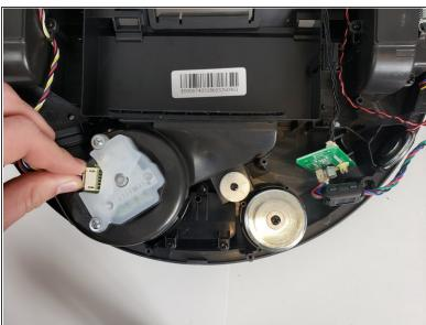
Carefully lift the laser unit off of the motor assembly.
