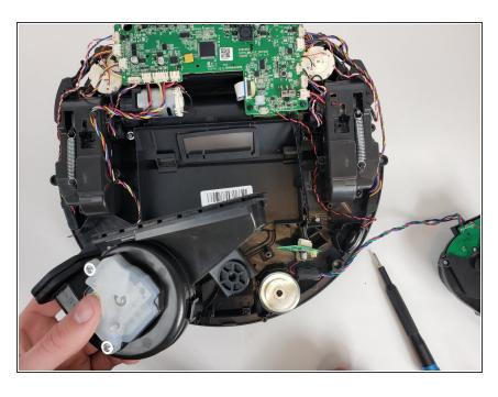
Lift and remove the motor assembly out of the Deebot. To reassemble your device, follow these instructions in reverse order.
