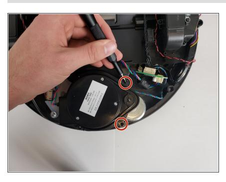
Using the Phillips #00 screwdriver, remove the three screws around the laser unit.
