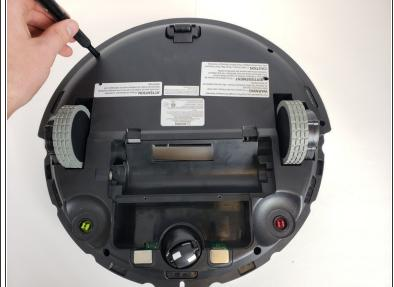
• Using a Phillips #00 screwdriver, remove the eight screws on the bottom edge of the bumper.
