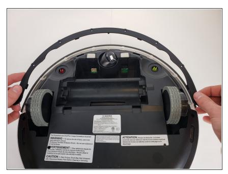
Remove the black strip on the bottom of the bumper.
