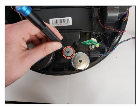
Remove the single screw holding the motor assembly in place using the Phillips #00 screwdriver.
