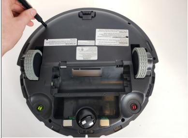
• Using a Phillips #00 screwdriver, take out the six screws around the perimeter of the bottom case.
