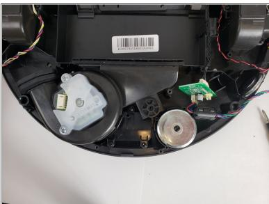
Disconnect the ribbon cable holding the assembly in place.
