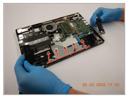
• Gently remove the connecting wire from underneath the wire brackets from the back of the computer.
