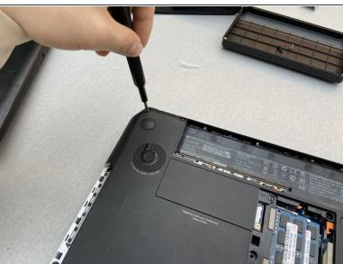
Remove the 13 screws on the bottom of the laptop that secure the top cover using a Phillips #1 screwdriver.
