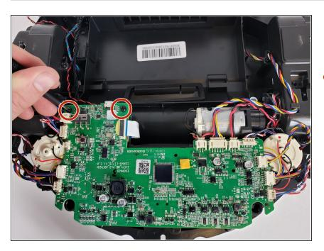
Using a Phillips #00 screwdriver, remove the two black screws holding the motherboard in place.
