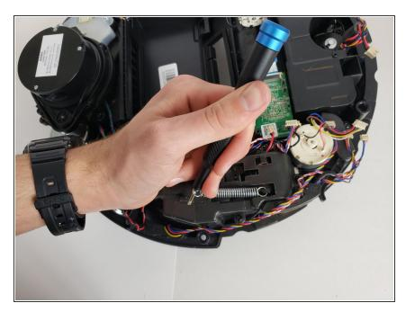
• Using a screwdriver or tweezers, remove the spring by lifting the spring and pulling it off one side.
