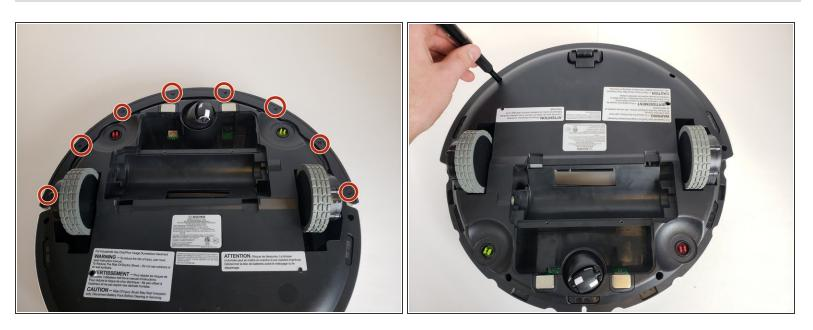
Using a Phillips #00 screwdriver, remove the eight screws on the bottom edge of the bumper.
