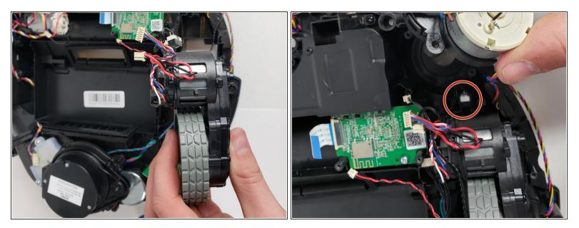
• Lift up and remove the wheel assembly and the attached sensor (black cable).
