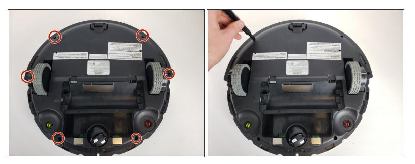
• Using a Phillips #00 screwdriver, take out the six screws around the perimeter of the bottom case.
