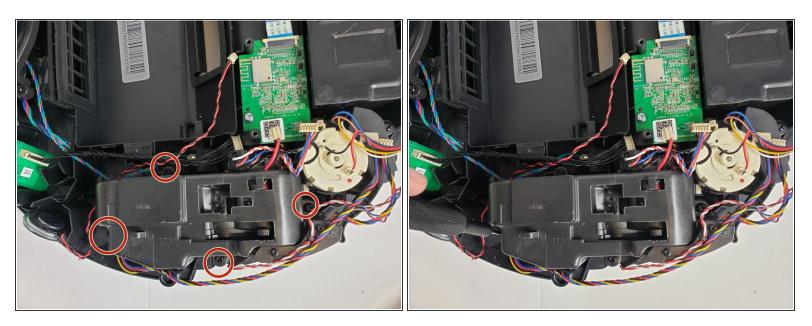
• Using a Phillips #00 screwdriver, remove the four screws holding the wheel assembly in place.
