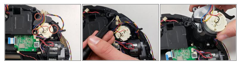
Using the Phillips #00 screwdriver, remove the three screws holding the side brush motor in place and lift the brush motor up.
