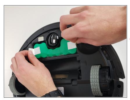
• Using the two white straps on the sides of the battery, gently remove the battery.
