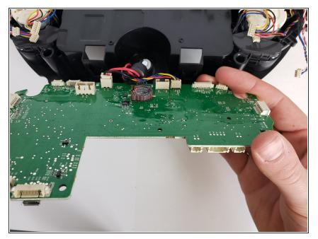
Remove the last three ribbon cables on the underside of the motherboard.
