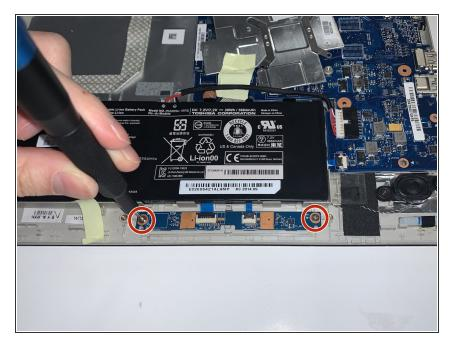
Remove any pieces of tape securing the board.
