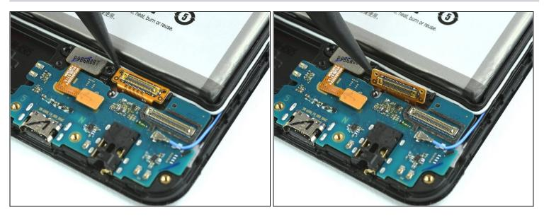
• Use the tip of a spudger to loosen the display connector above the daughterboard.
