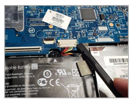
Pull the white cable connected to the motherboard out using the iFixit opening tool.
