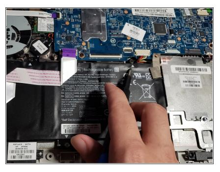
Using the Phillips #0 screwdriver, remove the five screws holding the battery in place.
