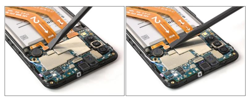
Use a spudger to disconnect the battery by prying the connector straight up from its socket.
