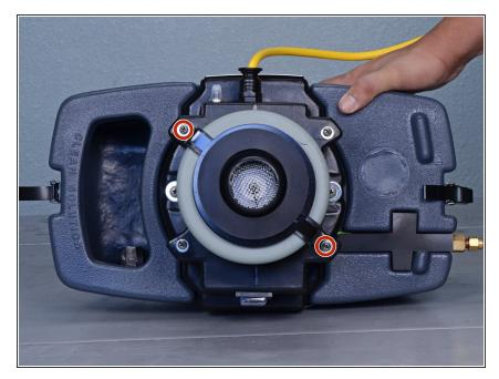
Use a Phillips #2 screwdriver to remove the two 1/2" screws and washers securing the vacuum motor retainer.
