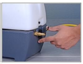
Unclasp and release the two black latches on either side of the carpet extractor.
