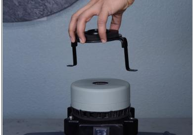
• Remove the vacuum motor cover, retainer, and gasket as one piece.
