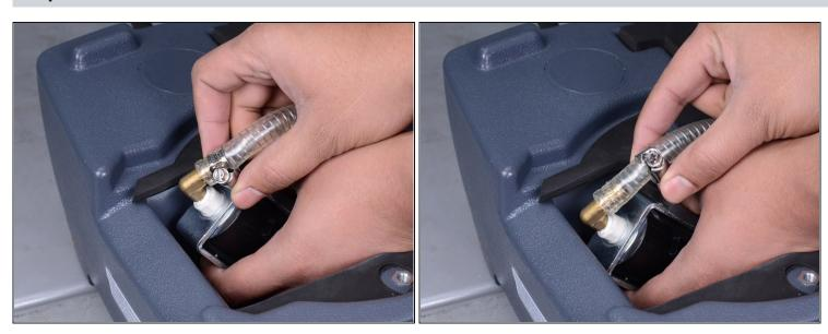
Slide the loosened hose clamp back until it is no longer around the brass fitting.
