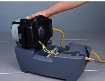
• Tilt the vacuum motor and pump housing sideways and let it rest on the side of the extractor.
