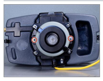
Use a Phillips #3 screwdriver to remove the two 1-1/2" screws and washers securing the pump housing.
