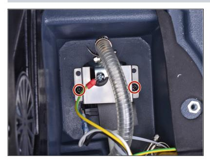
Use a Phillips #2 screwdriver to remove the two 1/2" screws and star washers securing the pump mounting bracket.
