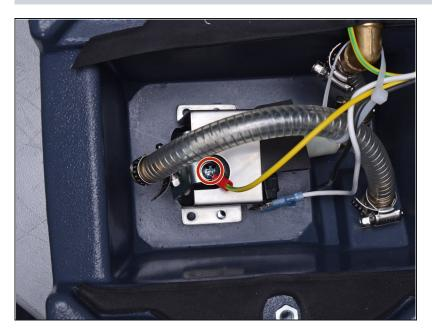
Use a Phillips #2 screwdriver to remove the ground terminal screw and star washer from the pump.
