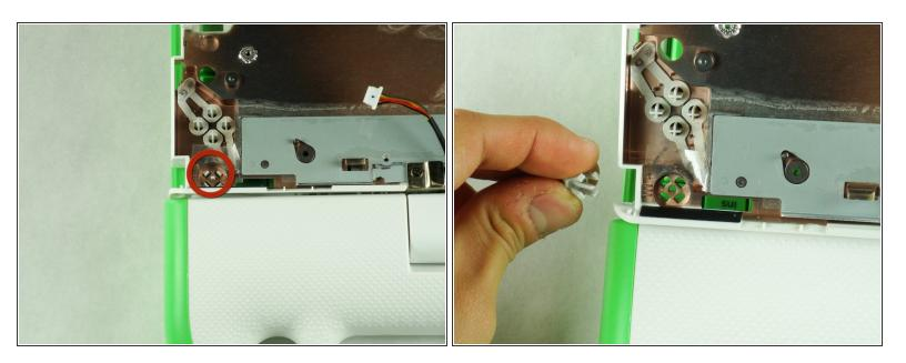
• Remove the power button by pinching in the four tabs until the power button can be pushed out.
