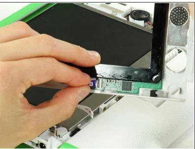
Lift the black connector and pull the ribbon cable out by the purple tab, freeing the frame.
