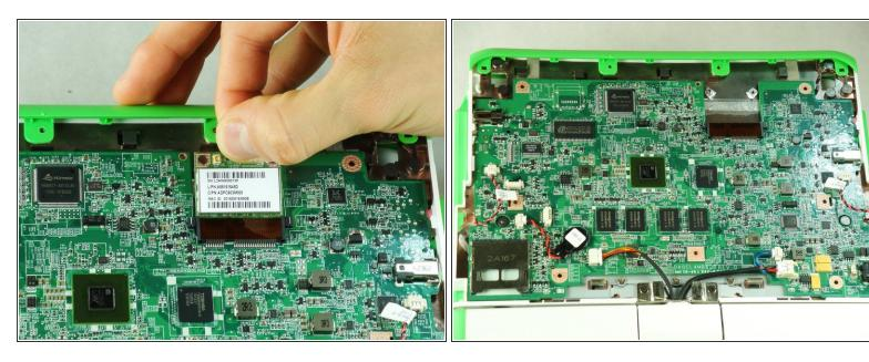
Remove the wireless card from the laptop by gently sliding it out of its socket.
