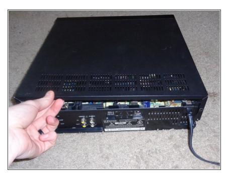
Lift up on the back case and slide the top case back until it is free from the rest of the case
