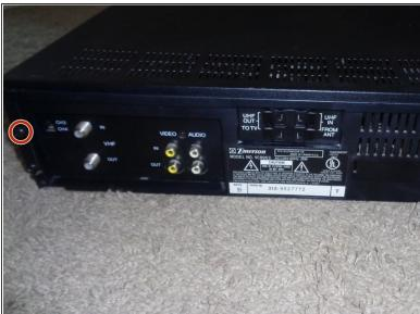
Remove the two 1/2" long #2 Philips screws from the rear of the case
