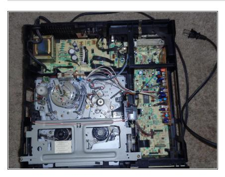
You will now have access to all the circuit boards and the top of all mechanical parts.
