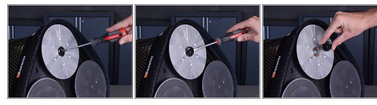
Use a flathead screwdriver to pry off and remove the rubber plug in the center of the sanding disc.
