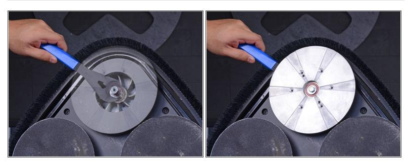
Slide a thin 22 mm wrench underneath the sanding disc and clasp it onto the flat part of the motor driveshaft to keep the driveshaft from turning.
