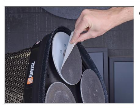
Peel the hook-and-loop sandpaper disc off of the driver assembly.
