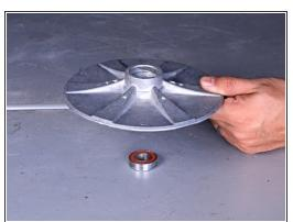
Place a 15/16" socket inside the center of the sanding disc and use a mallet to tap the bearing out of the disc.
