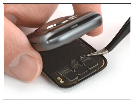
• Use a pair of tweezers to carefully peel off the tape covering the three display cable connectors.
