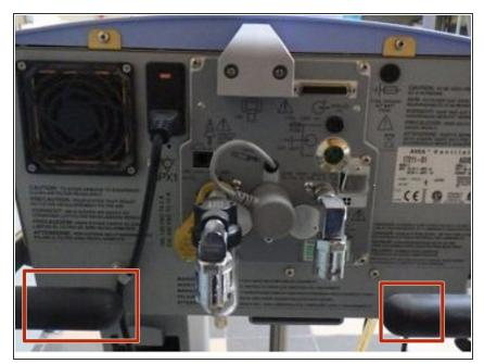
Remove the 'rubber collar' located at the UIM rear neck, by grasping one of the two rubber tabs at the bottom.
