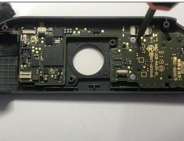
• Using a Phillips #2 screwdriver, remove the two 1.5 mm screws holding the motherboard in place.
