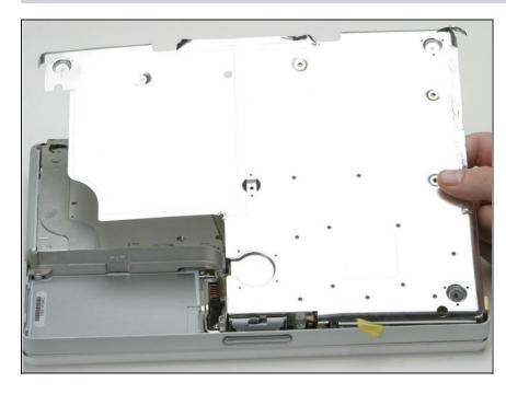
• Lift the bottom shield off.
