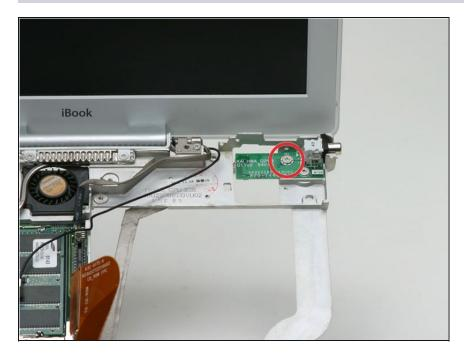
Remove the single 5.5 mm Phillips screw securing the DC-In board to the metal framework.
