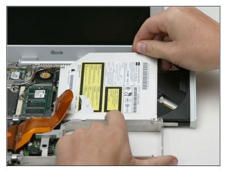
Lift the optical drive by the edge closest to the screen, minding that the metal bracket at the top left corner doesn't catch on the Airport or inverter cables.
