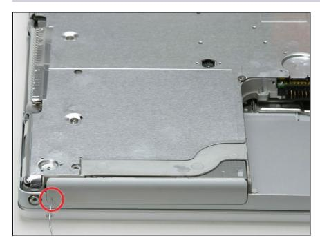
• Use a straightened paperclip to open the optical drive tray.
