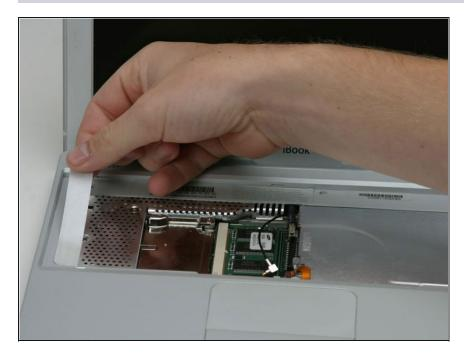
Peel up the foil tape covering the speaker cable near the ports.
