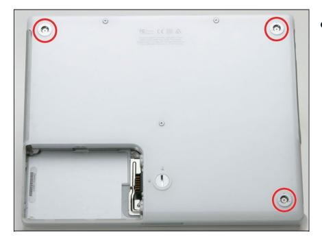
• Remove the three 5.2 mm newly-revealed Phillips screws.
