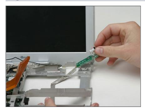
• Peel up the DC-In cable from the bottom of the metal framework and pull it through the conveniently-located nearby hole.
