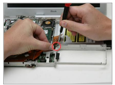
Peel back the orange ribbon cable to reveal a single Phillips screw.
