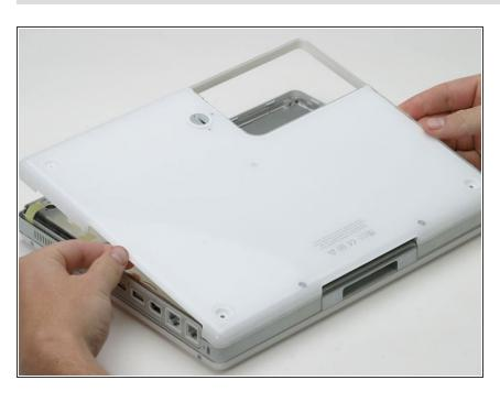
Once the front and sides of the lower case are free, turn the computer so that the back is facing you and pull the lower case up and toward you until the back tabs pop free (it may be helpful to jiggle the case up and down).
