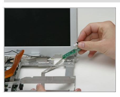
Peel up the DC-In cable from the bottom of the metal framework and pull it through the convenientlylocated nearby hole.
