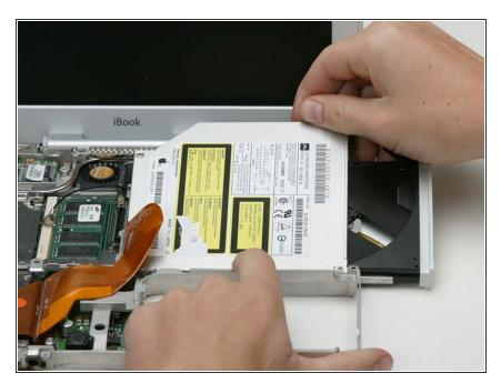
Lift the optical drive by the edge closest to the screen, minding that the metal bracket at the top left corner doesn't catch on the Airport or inverter cables.
