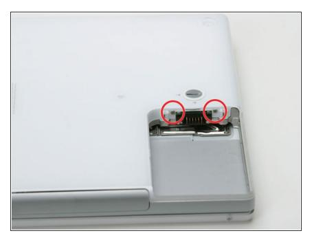
Remove the two 4.2 mm Phillips screws on either side of the battery contacts.
