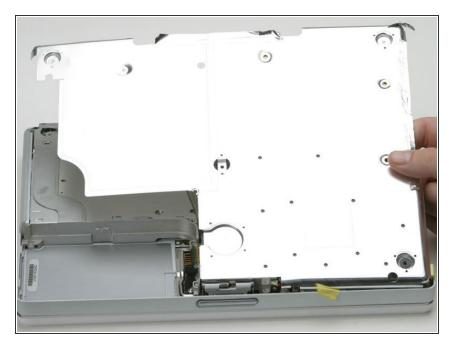
Lift the bottom shield off.
