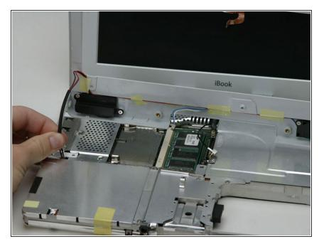
Lift the upper case off completely and disconnect the red and black speaker cable from the logic board.
