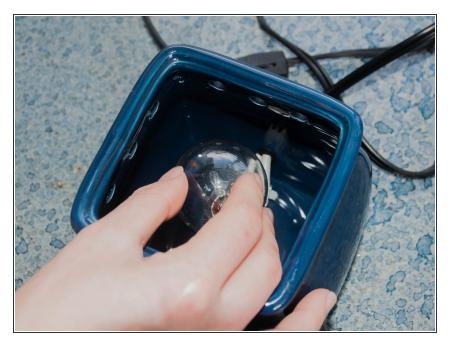
Screw in the new light bulb in a clockwise direction.
