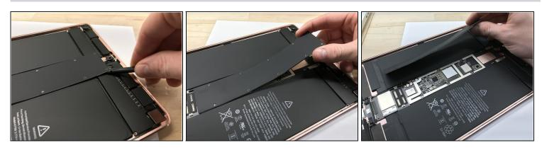
• Remove the logic board shield
