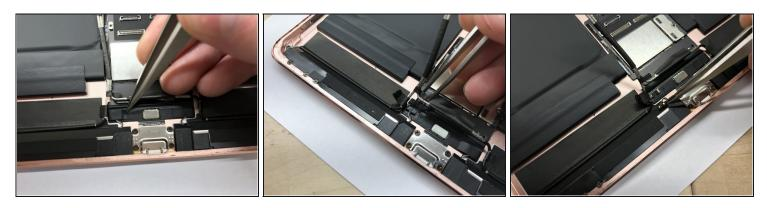
• Pull back on the tape covering the speaker FPC and disconnect the FPC.
