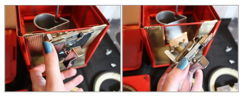
Remove the inner mechanism by pulling out one side before sliding out the whole mechanism.
