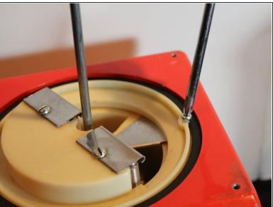
Using a Phillips #1 screwdriver remove the two 15mm screws that are marked in the photo.
