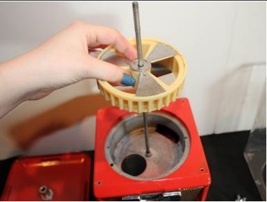
Remove the inner mechanisms by sliding them up and off the metal rod.
