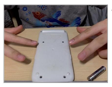
Remove 6 Philips screw to take the cover off.
