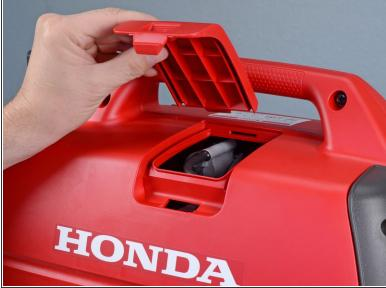
Lift and remove the spark plug cover.
