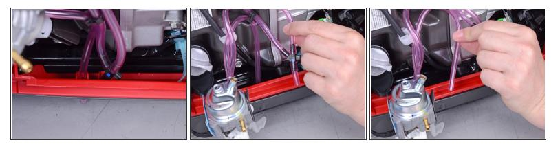
Pull the air vent tube and drain tube out of the port holes on the bottom of the cover.
