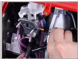
Pry and disconnect the fuel hose from the carburetor intake.
