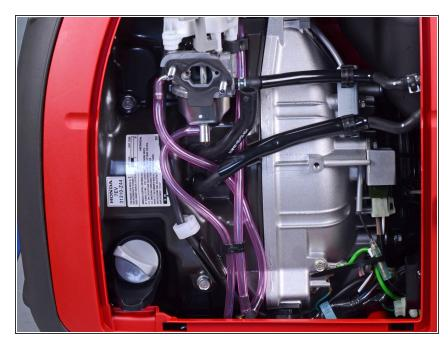
During reassembly, use this photo as a reference for how to route the tubing.
