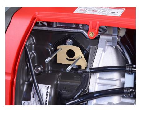
Replace the carburetor seal if it shows signs of wear. To reassemble your device, follow these instructions in reverse order.
