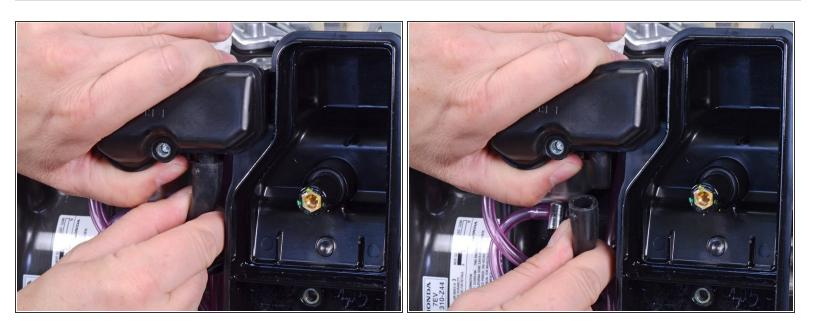
Disconnect the breather tube from the air cleaner housing.
