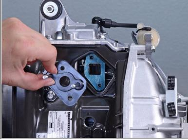
Remove the carburetor insulator along with the two bolt rails.
