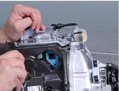
Begin separating the right shroud from the engine assembly by pulling it away from the assembly.
