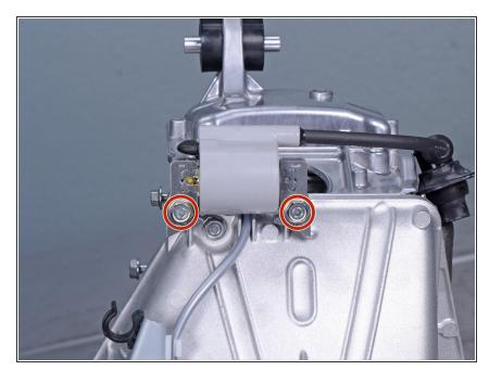
Use a 10 mm socket to remove the two bolts securing the coil ignition assembly.
