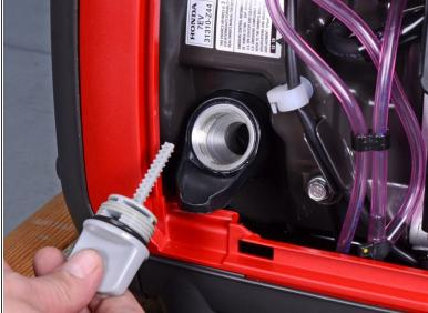
Unscrew and remove the oil filler cap.
