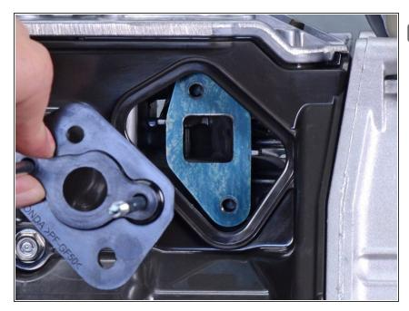
During reassembly, replace the insulator gasket if it shows signs of wear.
