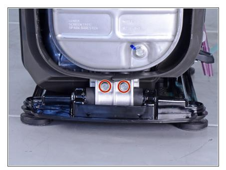
Use a 10 mm socket to remove the two bolts securing the motor rear to the under-cover.
