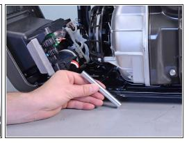
Use a mallet and punch to tap out the front collar (closest to the electrical panel) securing the motor assembly to the under-cover.
