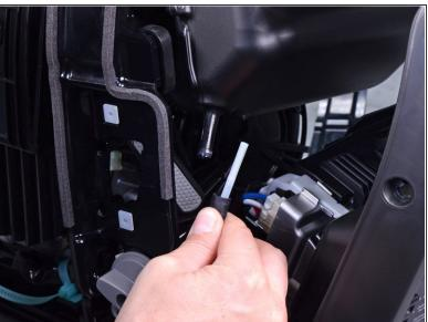
Disconnect the fuel line and filter from the fuel tank.
