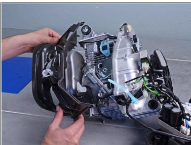
Remove the right shroud from the engine assembly.
