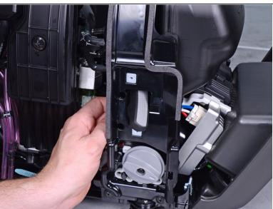
Feed the starter rope handle and guide through the panel cutout.
