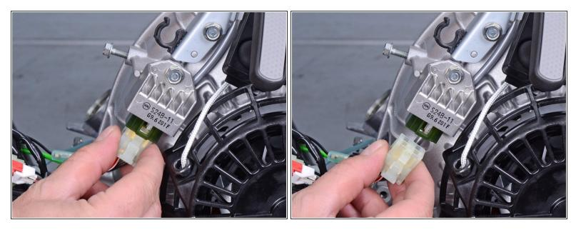
Disconnect the wiring harness from the rectifier socket.
