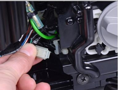
Pull and disconnect the engine stop switch connector from its socket.
