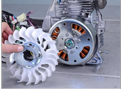
Remove the cooling fan, fan set plate, and starter pulley.
