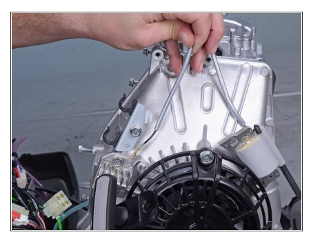
Remove the coil ignition assembly.
