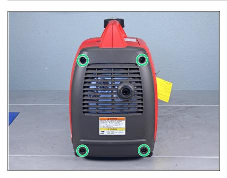
Remove the four Phillips screws securing the back cover.
