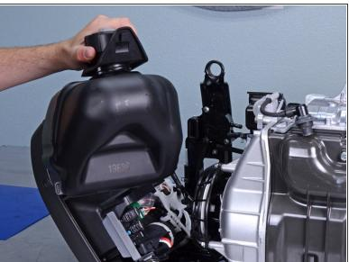
Lift and remove the fuel tank.
