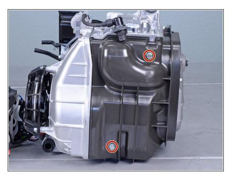
• Use a 10 mm socket to remove the two bolts securing the left shroud.
