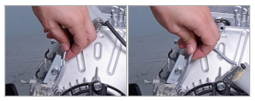
• Unroute the coil ignition wire from the engine assembly.
