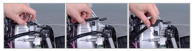
• Unclip the fuel and air hoses from the side of the motor assembly.
