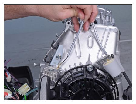
• Remove the coil ignition assembly.
