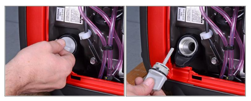
• Unscrew and remove the oil filler cap.
