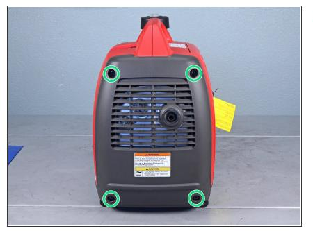
Remove the four Phillips screws securing the back cover.
