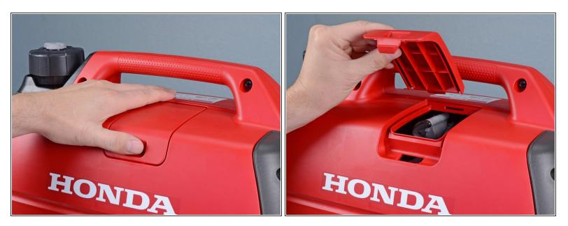
• Lift and remove the spark plug cover.
