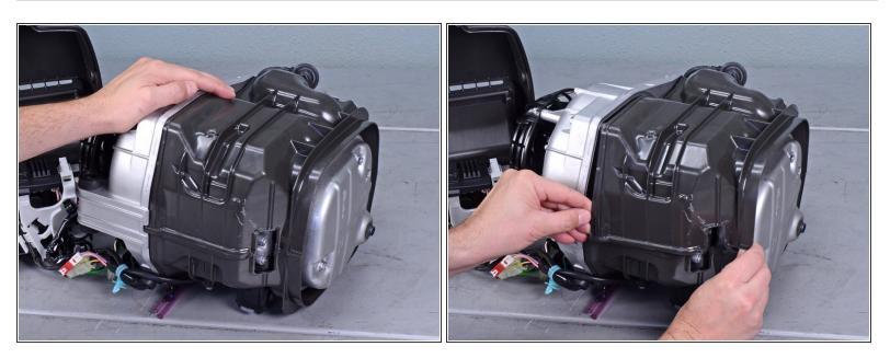
Begin separating the left shroud from the engine assembly by pulling it away from the assembly.
