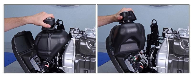
• Lift and remove the fuel tank.
