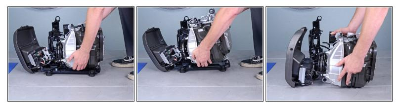
The motor assembly is heavy. Follow safe lifting practices when you lift the assembly.
