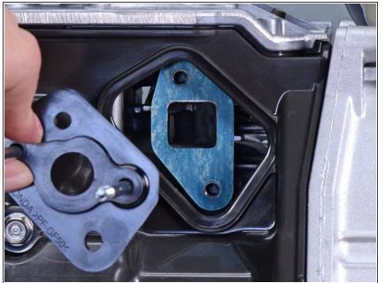
During reassembly, replace the insulator gasket if it shows signs of wear.
