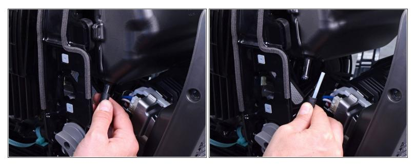
• Disconnect the fuel line and filter from the fuel tank.
