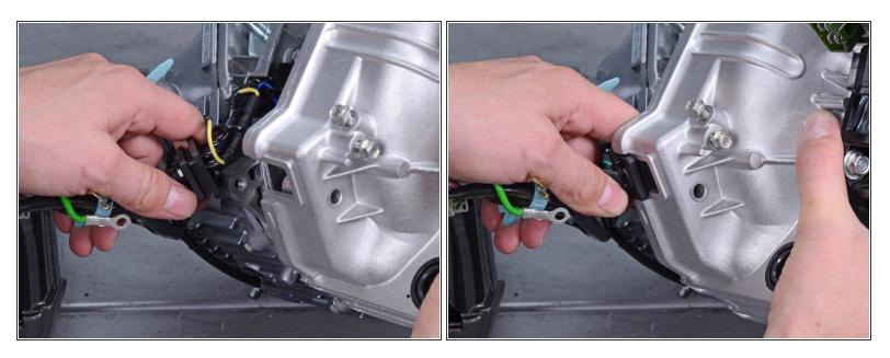
During reassembly, make sure that the cable strain relief sits properly in its fan cover cutout.
