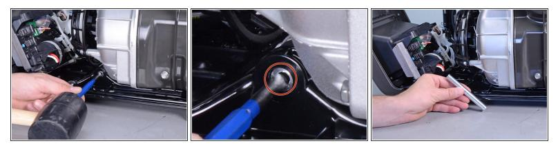
Use a mallet and punch to tap out the front collar (closest to the electrical panel) securing the motor assembly to the under-cover.
