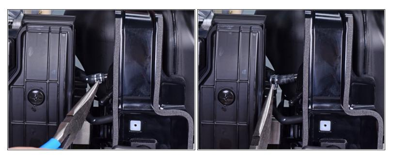
• Use a pair of pliers to squeeze and slide the spring clip off the fuel pump port.
