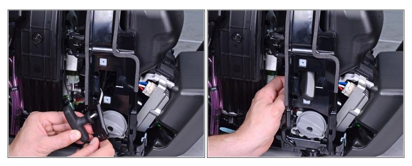
• Feed the starter rope handle and guide through the panel cutout.
