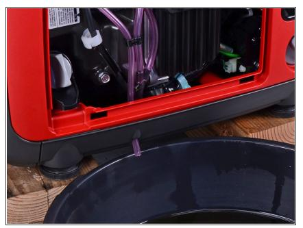
• Place a container below the drain tube to catch the excess fuel.
