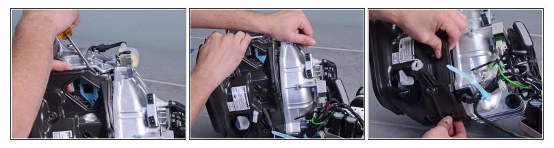
• Pull the shroud away along the edge. Use a flathead screwdriver to pry it out of the engine assembly groove.
