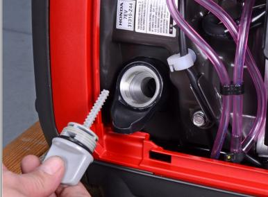
Unscrew and remove the oil filler cap.
